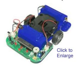
Ashley Mayes has made a Linbot which is a line-following robot manufactured by Active-Robots.
